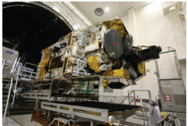
The first of Inmarsat’s I-6 satellites, I-6F1, which carries L-band and Ka-band payloads, so also is known as GX6A, enters thermal vacuum testing in Toulouse, France. Manufactured in the UK and assembled in France, I-6F1 undergoes this test to simulate the harsh space environment prior to launch in H2 2021.
